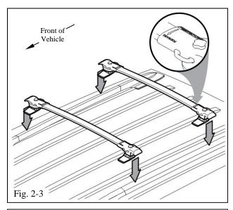
(d) Lower the crossbars between the roof rails (Fig. 2-3).
