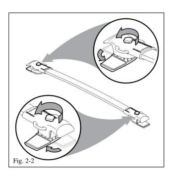
(b) Loosen the clamps by turning the knobs counterclockwise (Fig. 2-2).
